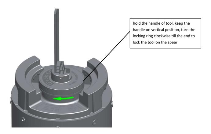
4. turn and pull down the handle of the tool for 90 degrees, release the pressure from the keg till no gas comes out from the keg
