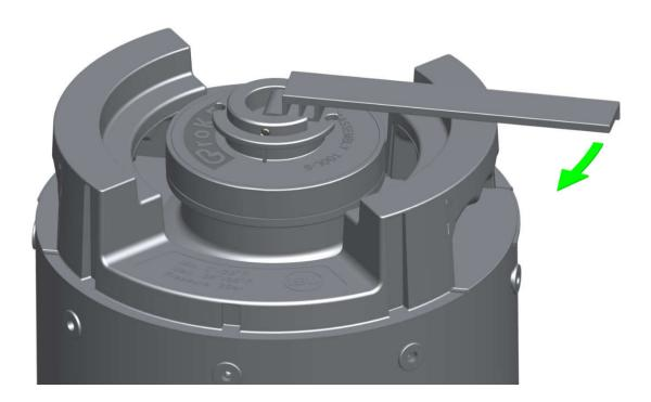
6. turn the locking ring of the tool anticlockwise till the end, to unlock the tool and take the tool off from the spear. The keg is ready for filling.
