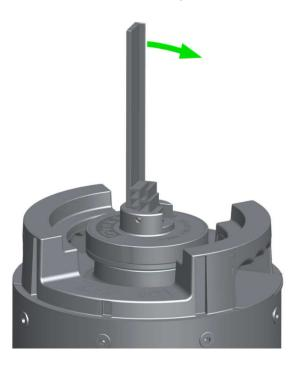
5. hold the handle of tool, turn the tool and spear clockwise till the spear screwed tightly on the keg
