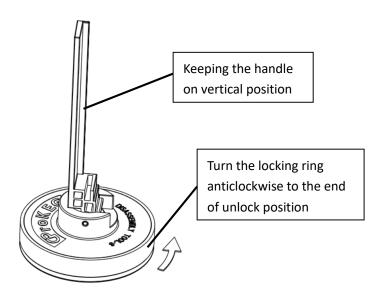
2. aligning the assembly/disassembly tool on the spear
