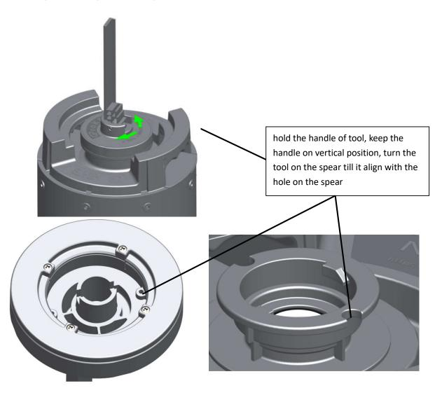
3. locking the assembly/disassembly tool on the spear
