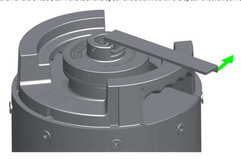
6. turn the locking ring of the tool anticlockwise till the end, to unlock the tool and take the tool off from the spear; pull the inner bag out from the keg.
