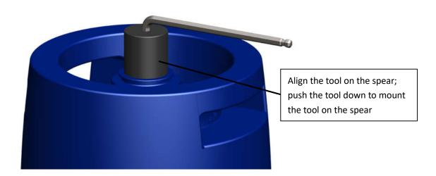
3. hold the key of tool, turn the tool and spear clockwise till the spear screwed tightly on the keg
