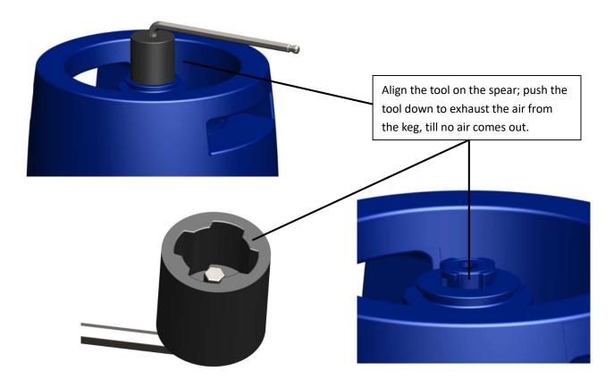
2. hold the key of tool, turn the tool and spear anticlockwise till the spear unscrewed from the keg
